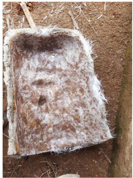
Plate 4: Positive Mold II, Concrete/Rice Husks/Resin/Fibre Matt, (30.2cm x 40.2cm),2025. Source: Researcher's Collection, Abakaliki, Ebonyi State, Nigeria
